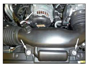
3. Remove the two bolts shown that secure the intake tube to the core support. Push the white locking tab for the crank case vent line down and then disconnect the crank case vent line from the intake tube.
